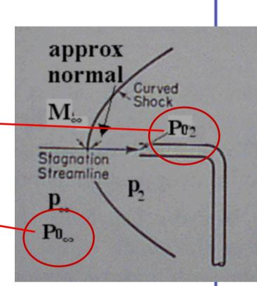
$$\frac{P_{02}}{P_{01}} = \frac{2}{(\gamma + 1)\left(\gamma M_1^2 - \frac{(\gamma - 1)}{2}\right)^{\frac{1}{\gamma - 1}}} \left(\frac{\left[\frac{(\gamma + 1)}{2}M_1\right]^2}{1 + \frac{(\gamma - 1)}{2}M_1^2}\right)^{\frac{(\gamma - 1)}{\gamma - 1}}$$
