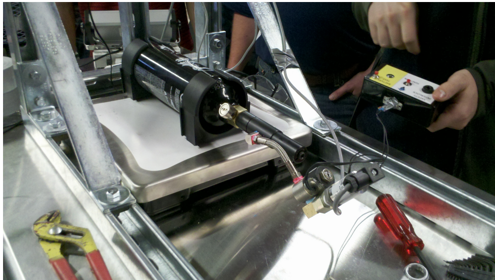
Figure 44: CO 2 output pressure calibration test.
