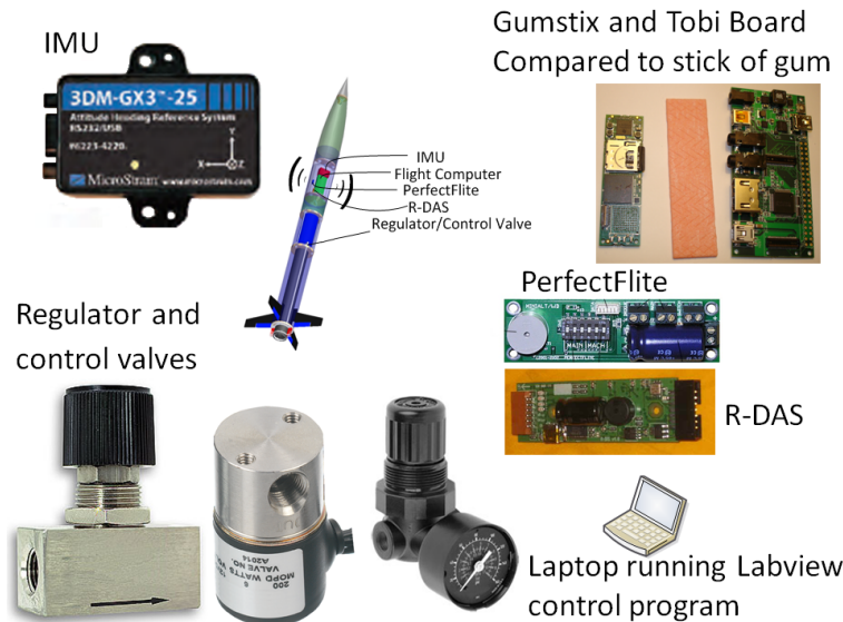
Figure 39: Avionics suite used for energy management algorithm and flight data management.
