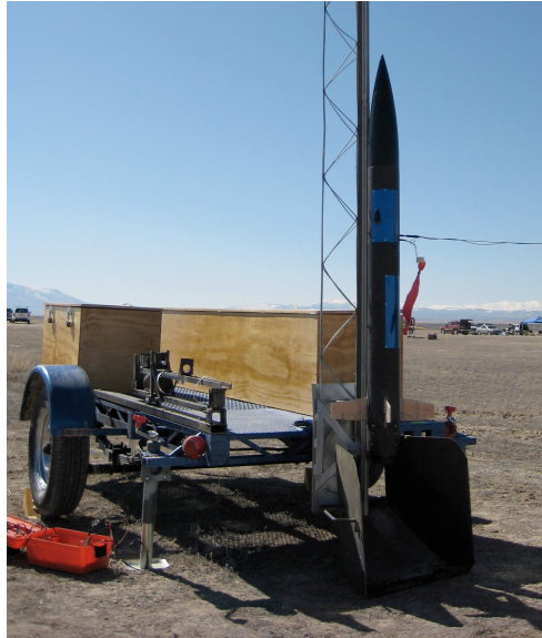
Figure 2: Chimaera mobile launch platform.
