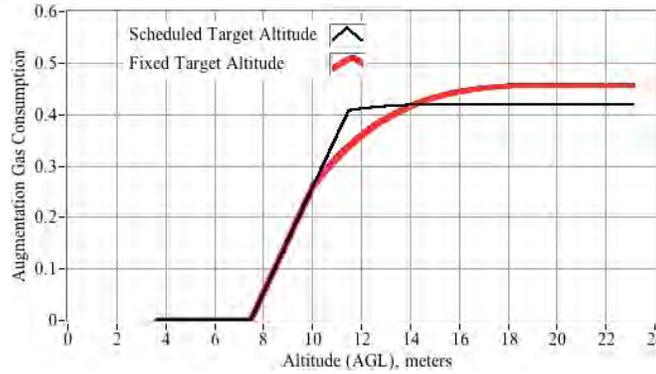
**Figure 8. Effect of Target Altitude Pre-Scheduling on CO<sub>2</sub> Propellant Consumption.**
