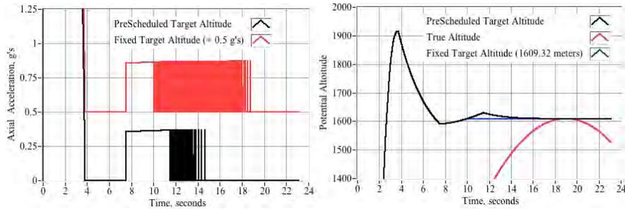
**Figure 7. Effect of Target Altitude PreScheduling on C-BAS Control Activity.**
