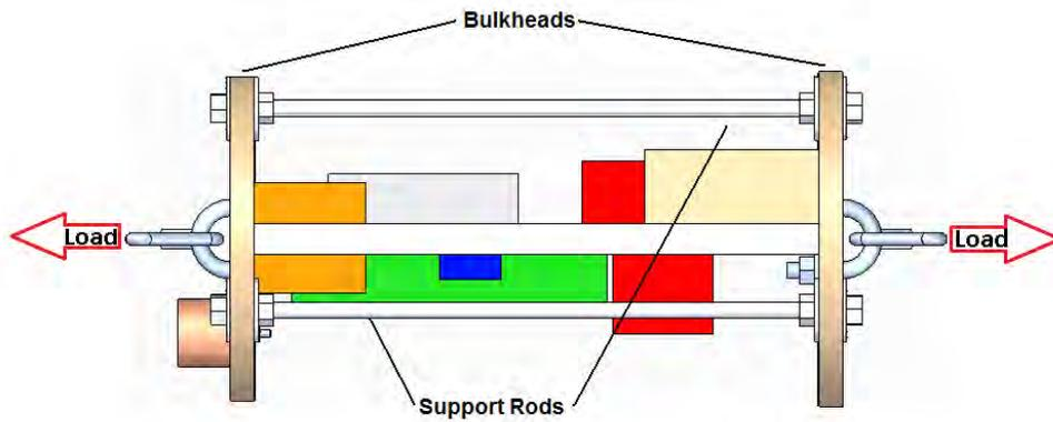
Figure 7: Avionics bay support rods.
