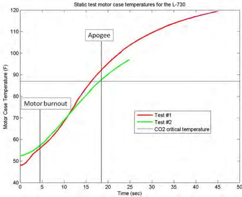
Figure 64: Static test motor tube temperatures.
