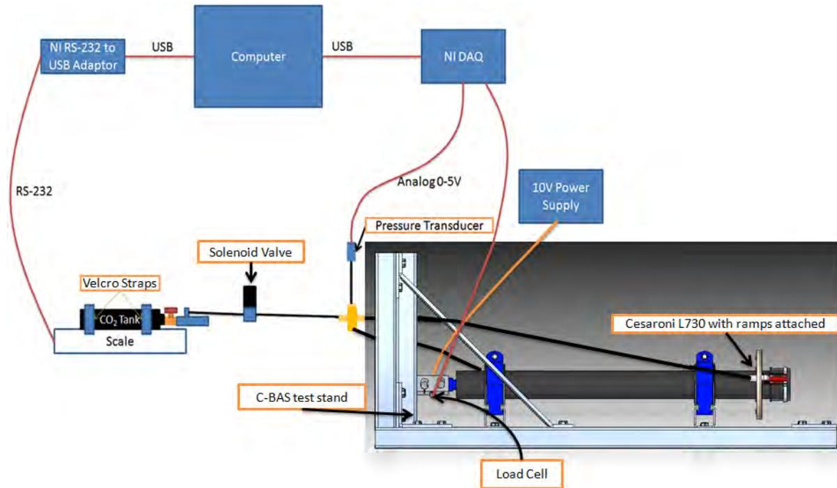
Figure 58: Cold gas test stand.
