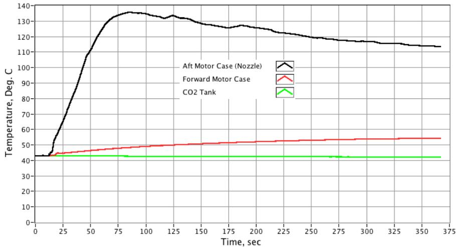
Figure 65: CTI L730 motor static test temperature profiles.
