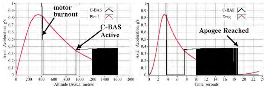
Figure 5. Comparison of the Vehicle Drag and C-BAS Acceleration Levels.
