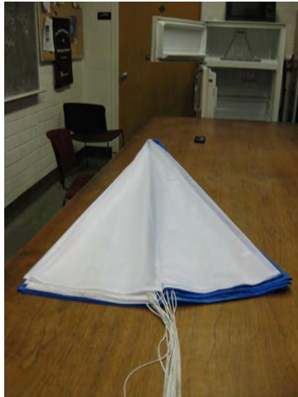
6. Open each flap to center. Fold over. Repeat for all flaps on one side; open; repeat folds for other side; open. Parachute should look like two accordions joined at the centerline. Consult pictures.
