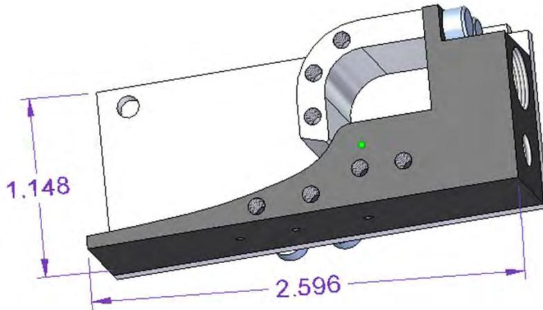
Figure 56: Solid model of the linear expansion ramps.
