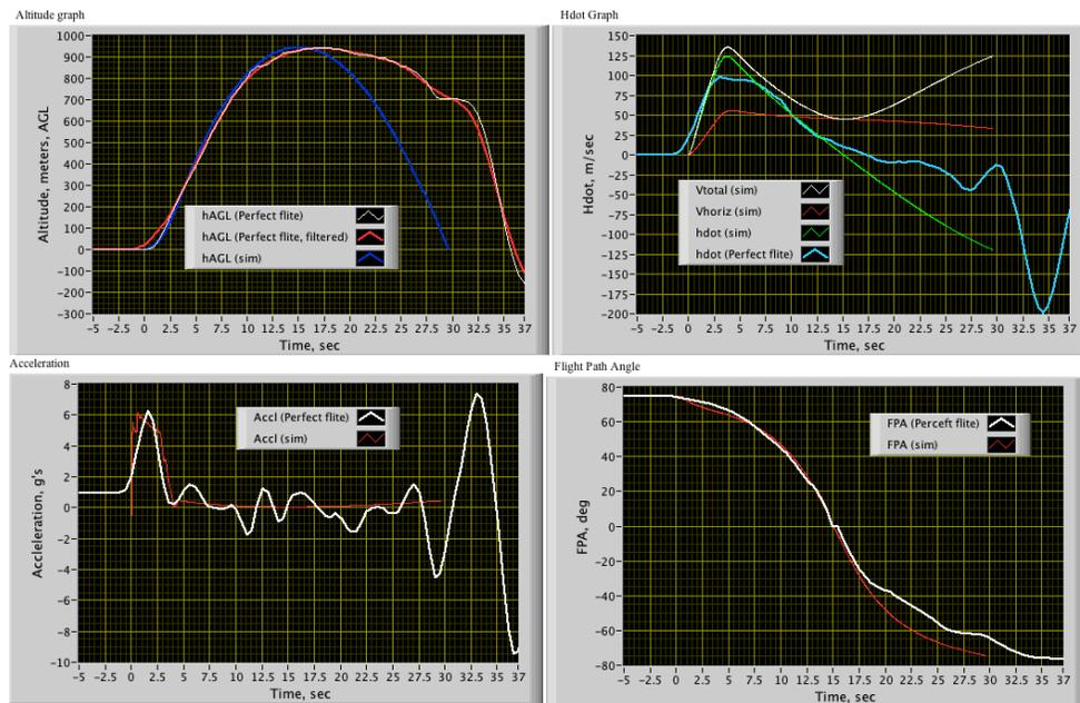
Figure 24: Flight data from the PerfectFlite altimeter.
