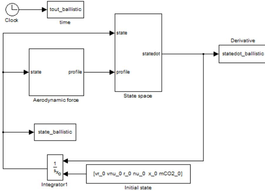
Figure 36: Rocket simulation model from MATLAB/Simulink.
