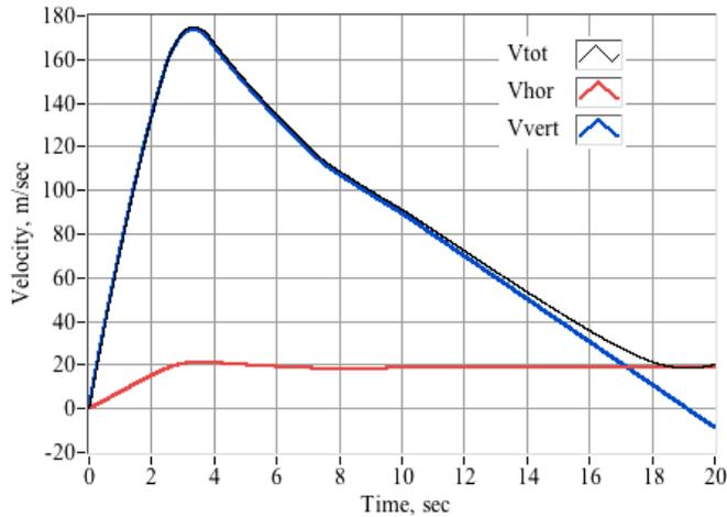
**Figure 3. Nominal Velocity Profile for CS -730 Launch**
