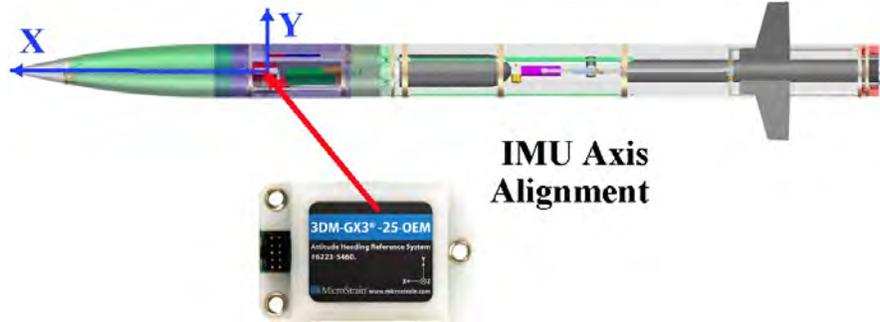
Figure 2. IMU Axis Orientation in Avionics Bay.
