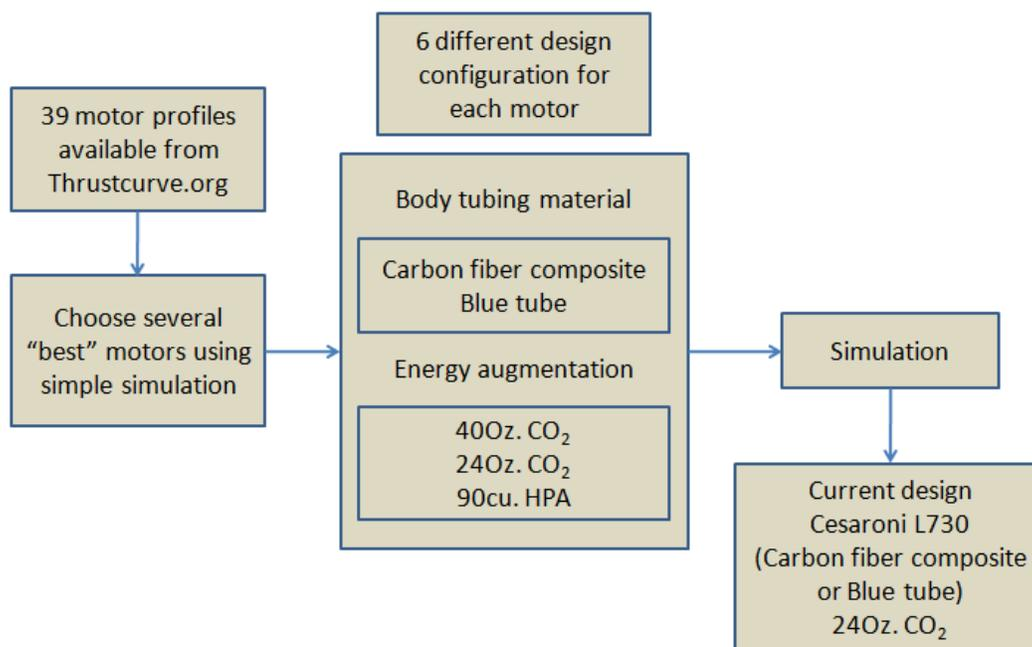
Figure 11: Motor and design selection procedure.
