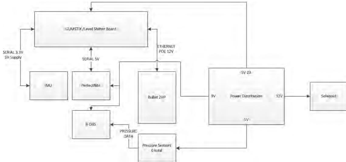
Figure 57: Block diagram of the avionics system.
