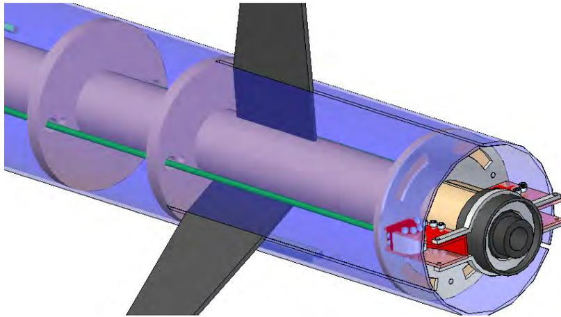
Figure 6: Integration of C-BAS expansion ramps into vehicle base area.
