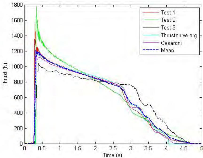
Figure 12: Cesaroni L730 test thrust data.
