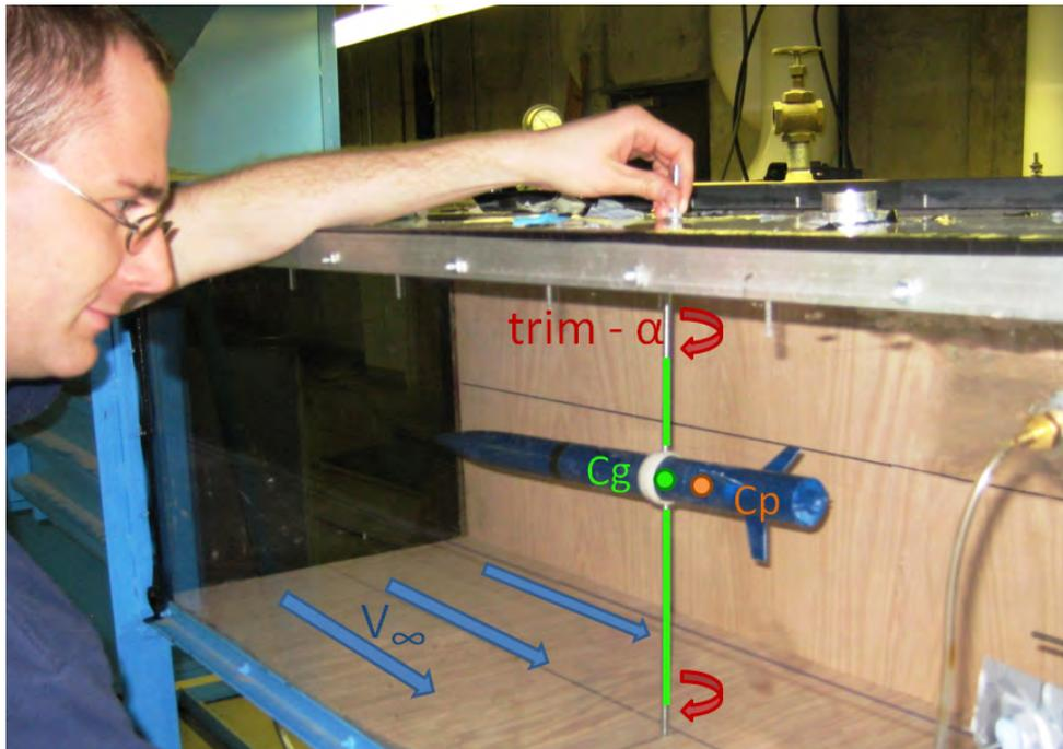
Figure 44: Test concept for  $C_P$  location and Javelin stability verification.
