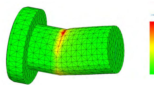
Figure 22: Finite element analysis on the screw
