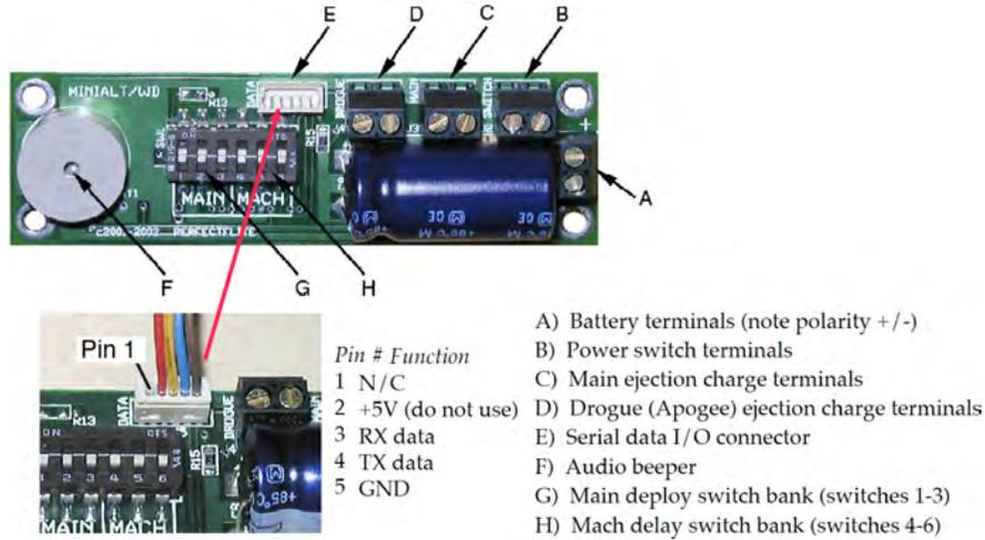
Figure 10 Major PerfectFlite Components and Serial I/O Connector Pinouts
