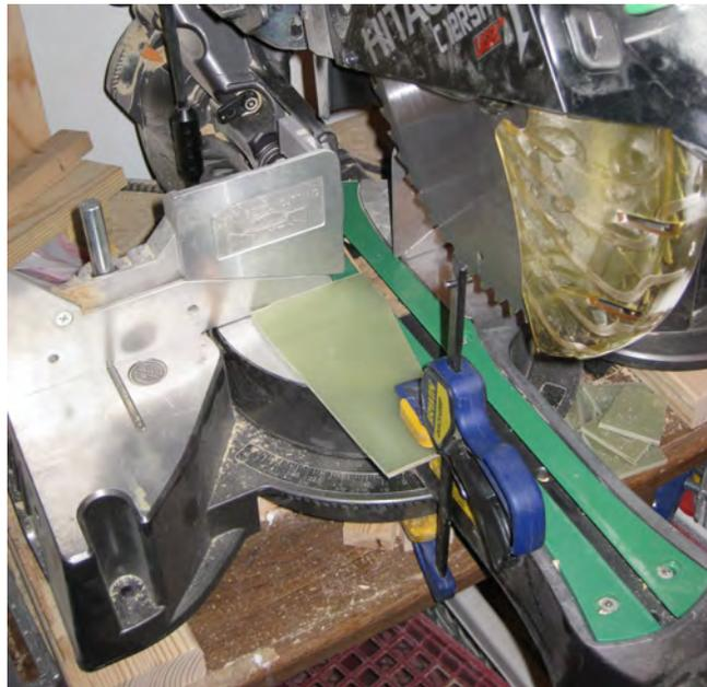
Figure 15: Miter saw and clamps used to cut fins
