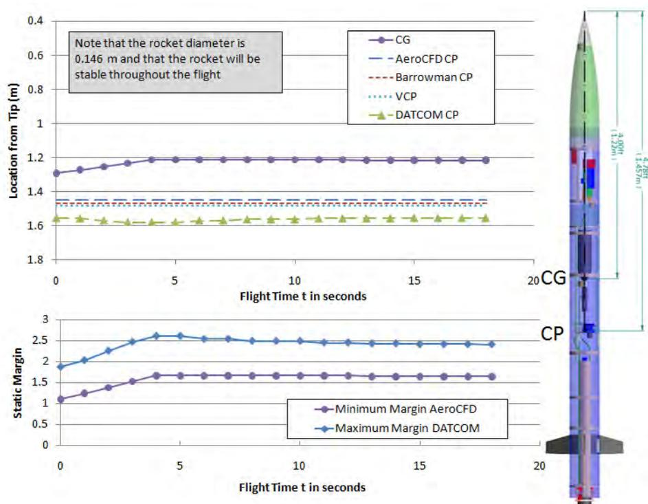
Figure 42: Center of mass and center of pressure over launch profile
