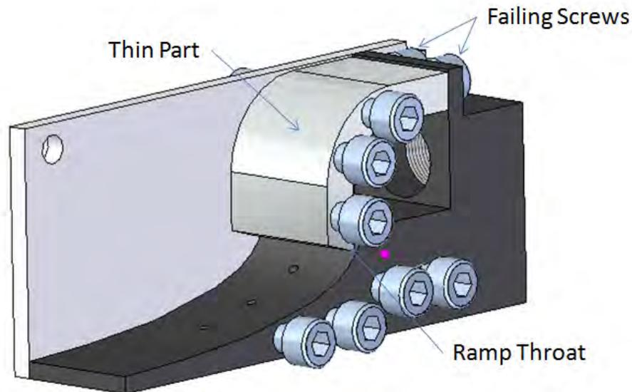
Figure 20: Ramps assembly with side plate removed.
