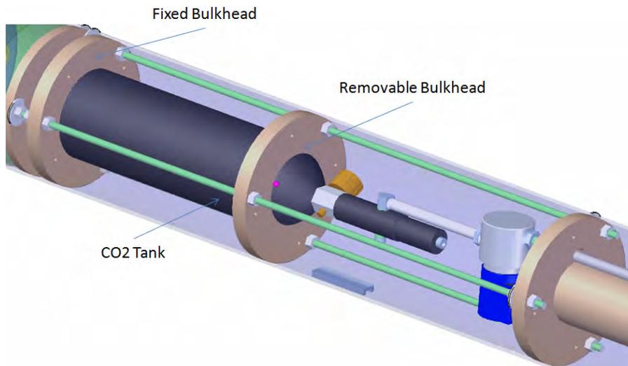
Figure 63: Supports for the CO<sub>2</sub> tanks.
