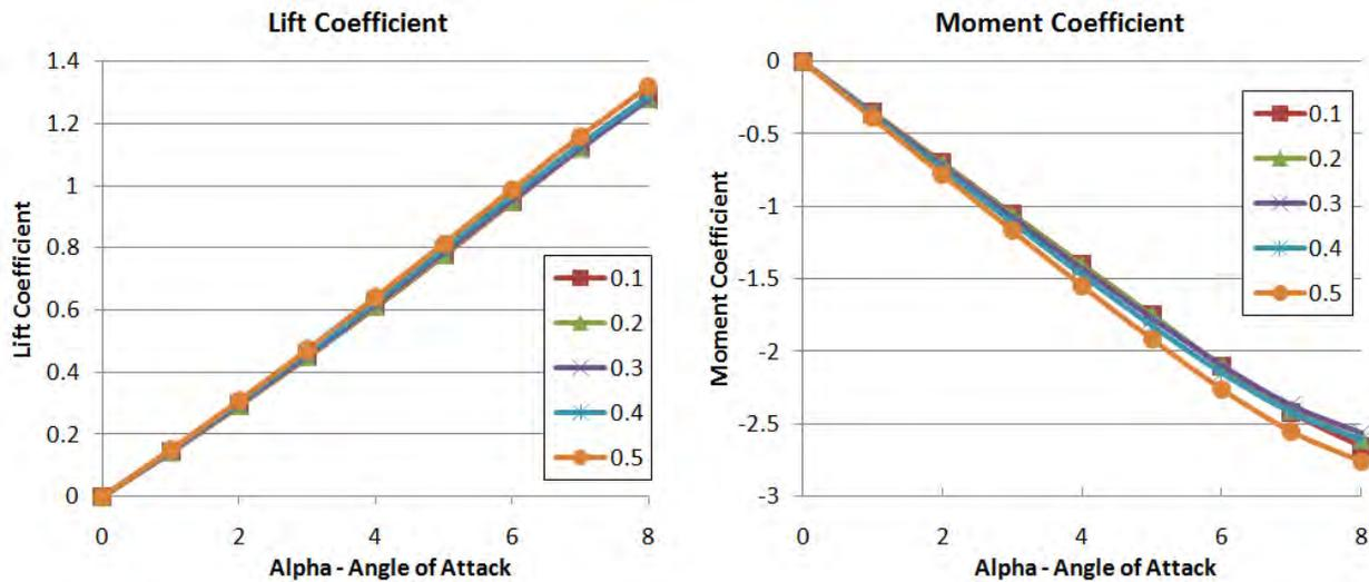
Figure 45: Missile DATCOM results for lift and moment coefficients.
