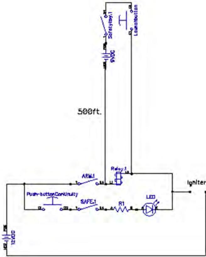
Figure 67: Launch controller wiring diagram.
