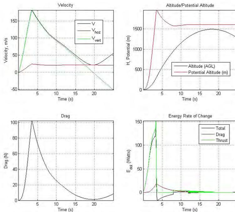
Figure 54: Unaugmented Javelin trajectories (C-BAS inactive).
