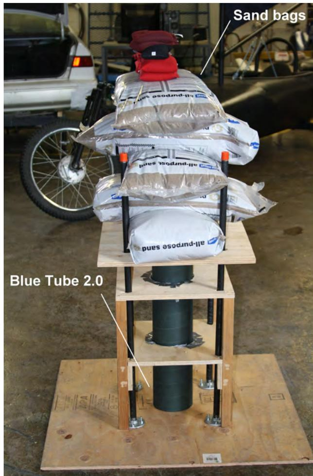
Figure 9: Body tube test stand.
