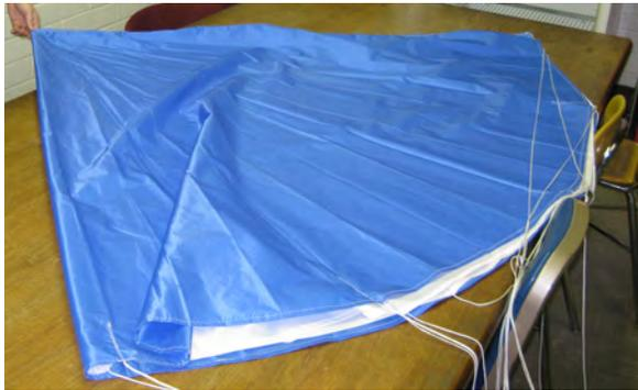
5. Fan panels over on top of each other until all lines are lined up from a center point. Open folds so that half are on each side of lines. The parachute should be shaped like an ice cream cone with shroud lines instead of an ice cream scoop.
