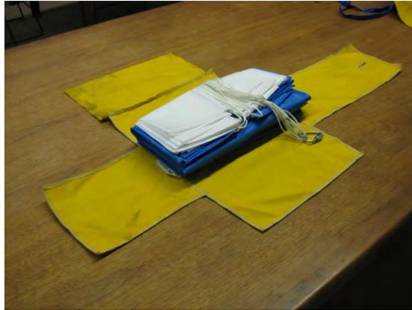
Parachute is ready for storage or packaging in rocket body. Perform this procedure after each parachute use.
