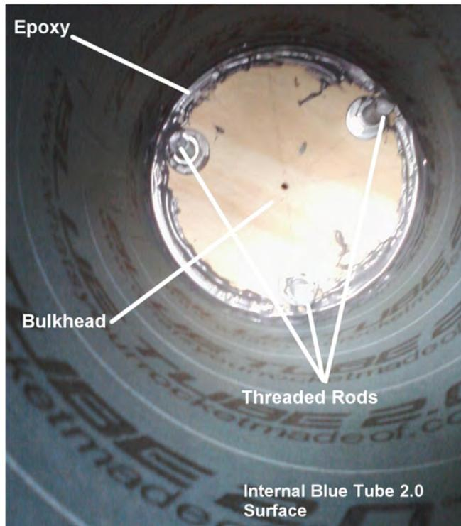
Figure 10: Bulkhead epoxied to the tube.
