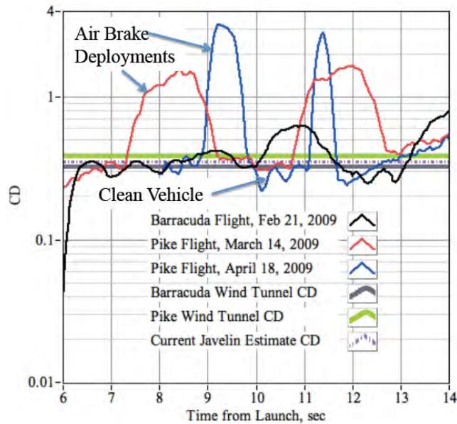
Figure 52: Drag coefficient comparisons of previously obtained flight data to current Javelin measurements.
