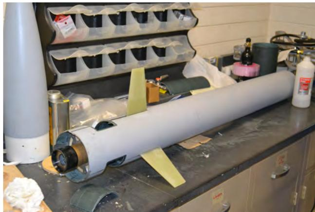
Figure 19: Finished fin assembly.
