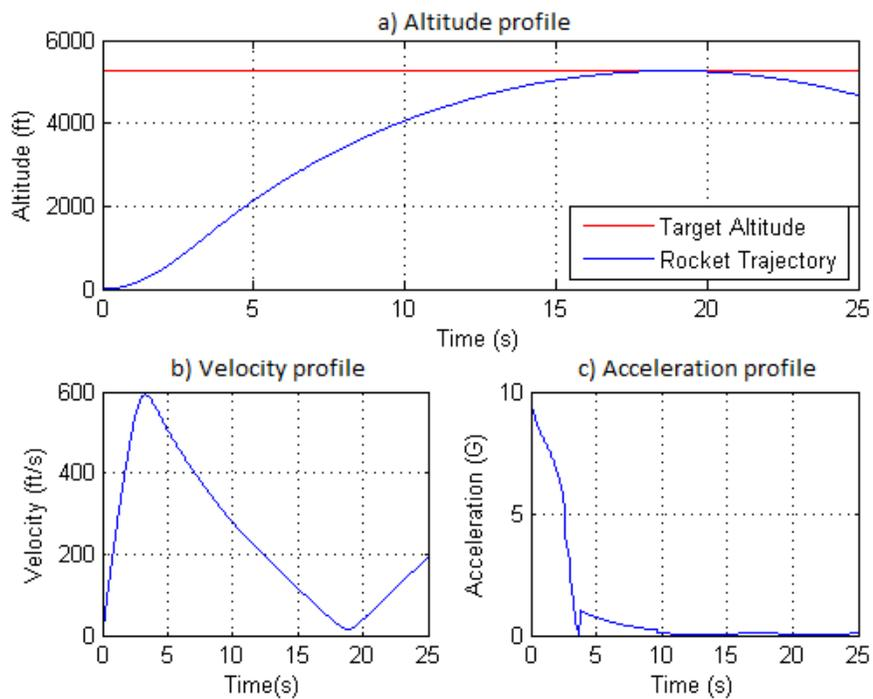
Figure 39: Rocket simulated trajectory with C-BAS active; a)Altitude, b)Velocity, c)Acceleration profiles.
