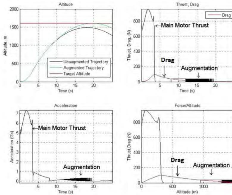
Figure 55: Augmented Javelin trajectory.(C-BAS active).
