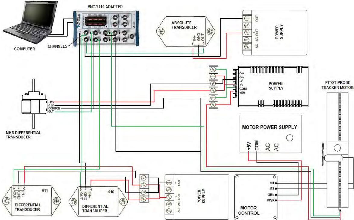
Figure 48: Wind tunnel hardware wiring diagram.
