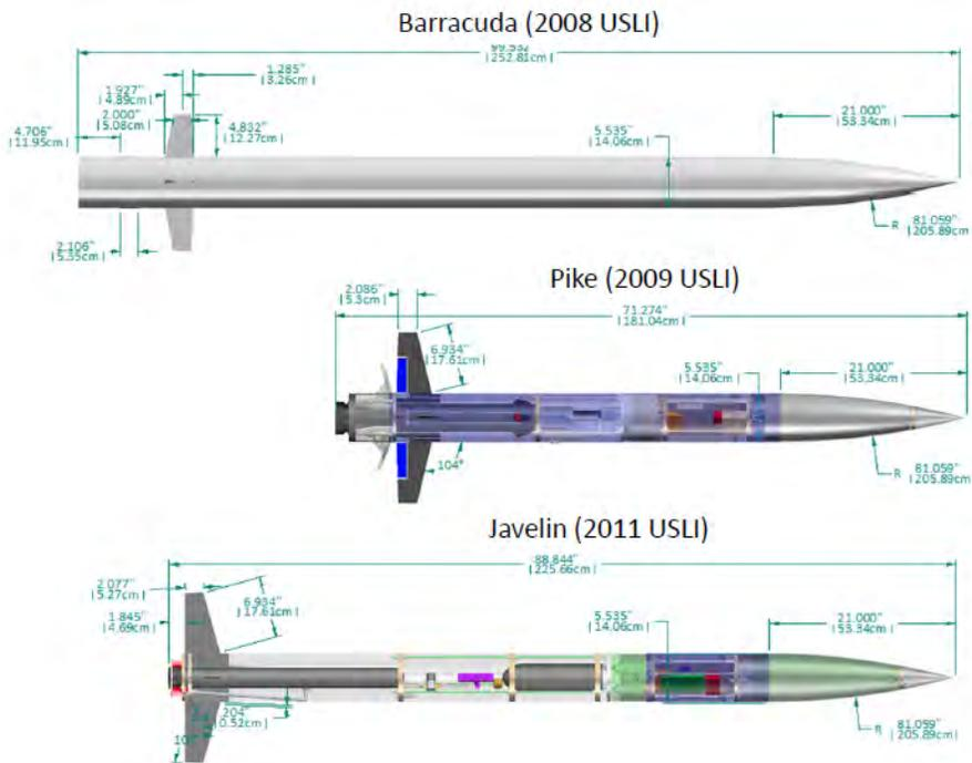
Figure 51: External mold-line comparison of the Javelin and previous USLI entries from Utah State.
