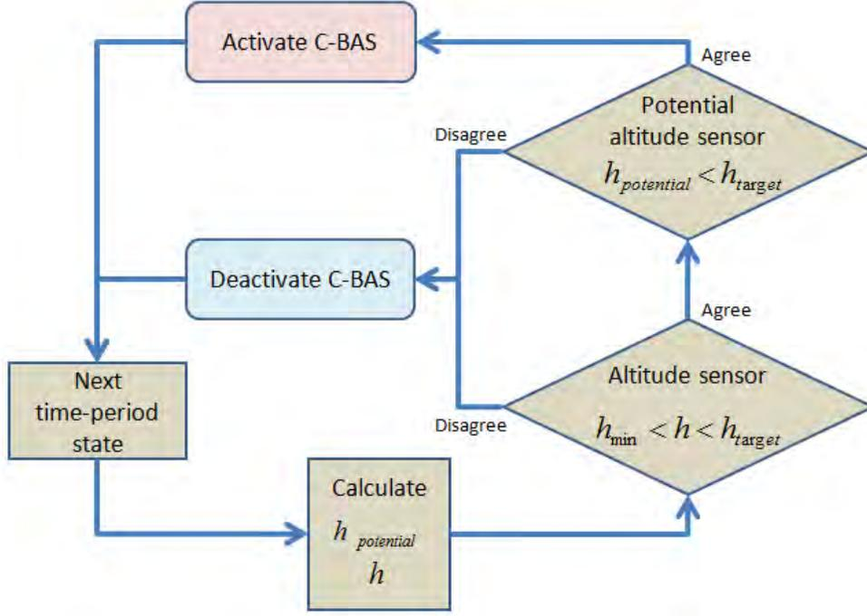
Figure 40: C-BAS algorithm for simulations.
