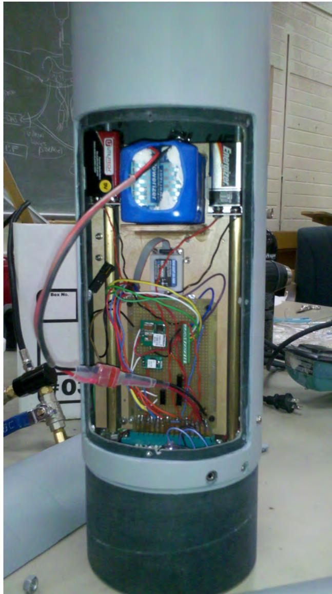
Figure 5: Access door in avionics suite.
