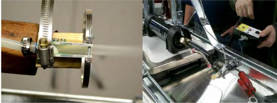
Figure 59: CO<sub>2</sub> output pressure calibration test.
