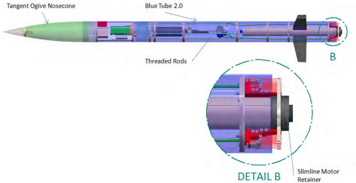
Figure 3: Vehicle structural layout.
