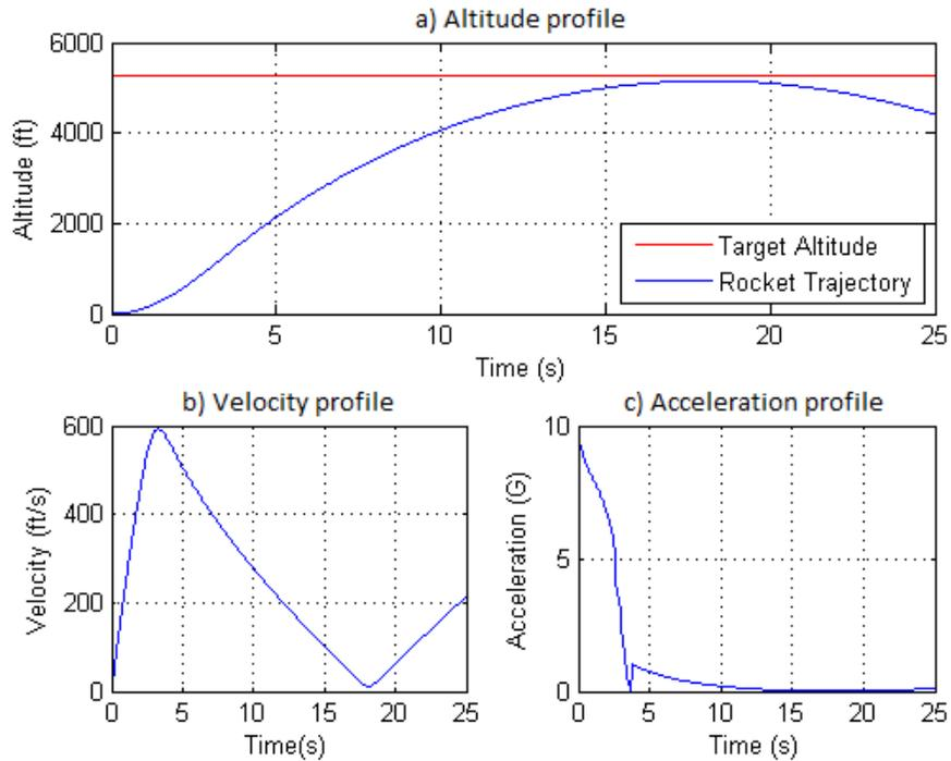
Figure 38: Rocket simulated trajectory with C-BAS inactive; a)Altitude, b)Velocity, c)Acceleration profiles.
