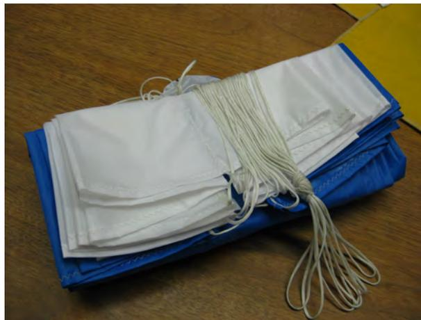
10. Secure carabineer to shroud line loop and attach harness at center loop. Place folded parachute in Nomex bag. Fold shroud line ends in figure 8 (or S) shape.
