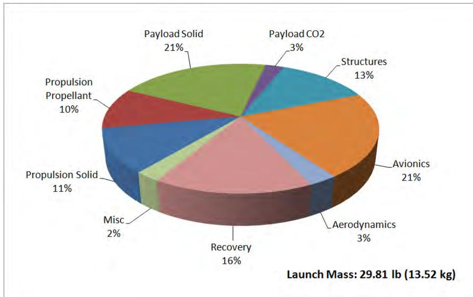
Figure 35: Projected vehicle mass breakdown.
