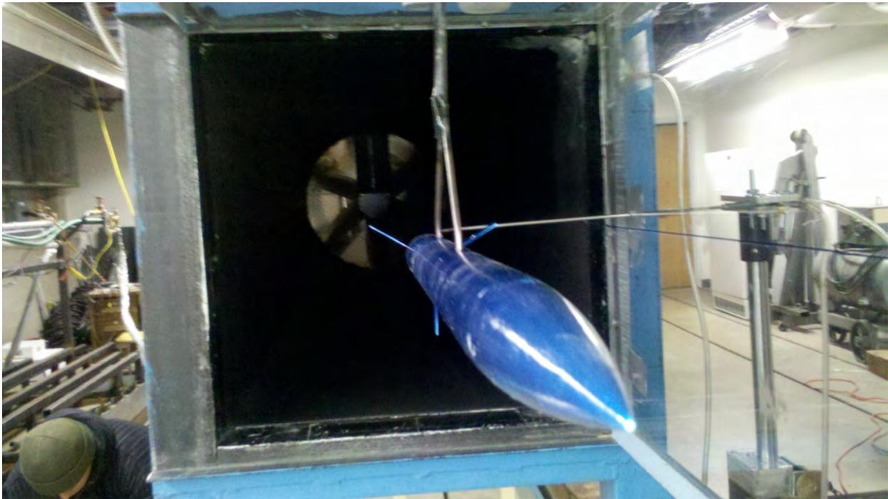
Figure 46: Dynamic view of Javelin model and pitot tube inside wind tunnel.
