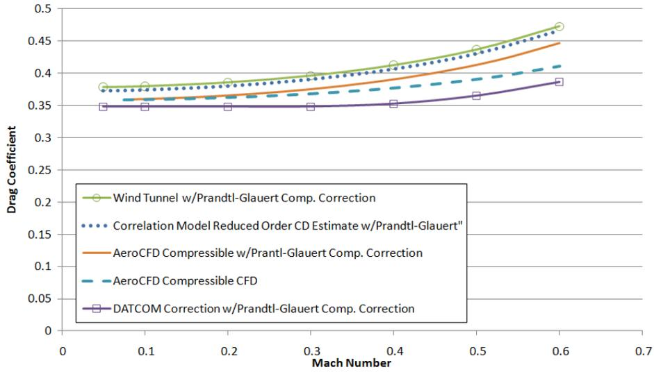
Figure 50:  $C_{D0}$  results comparison with compressibility correction.
