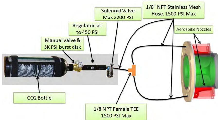
Figure 62: C-BAS component layout.
