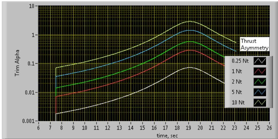
Figure 43: Plot of trim angle due to C-BAS thrust asymmetry.
