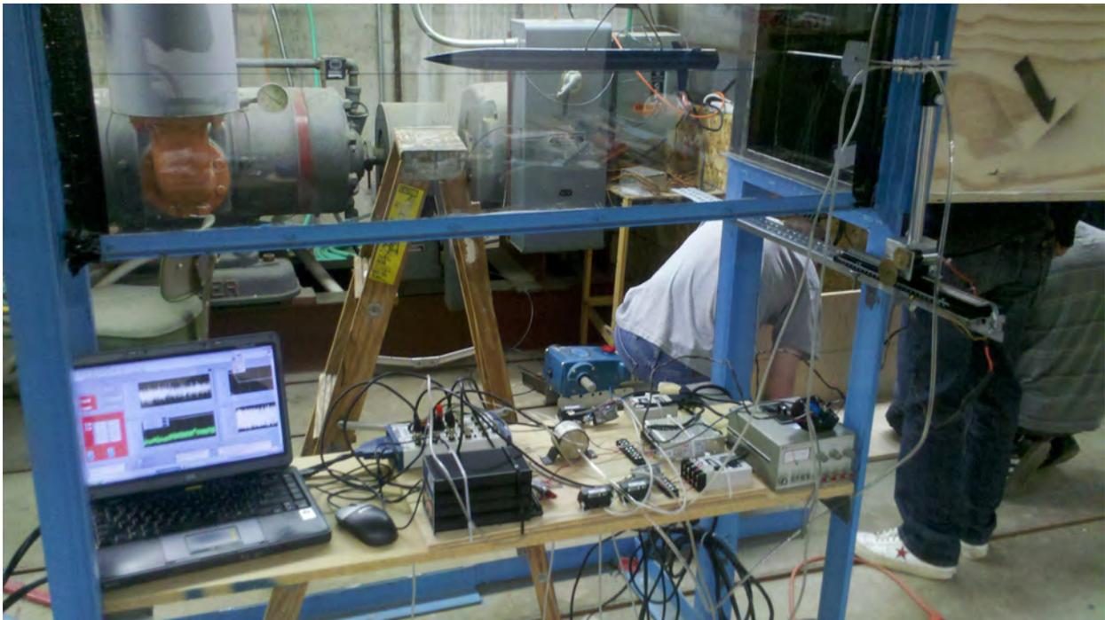
Figure 47: Wind tunnel wake survey hardware setup.
