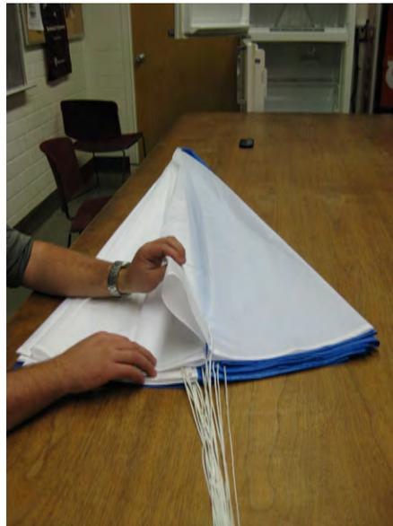
8. Lay shroud lines back on parachute. Loop at tip and bring back to base so that the loop, knot, and a couple of inches of line are left lying off of the parachute.
