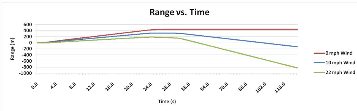
Figure 33: Landing footprint approximation for fixed wind speed.
