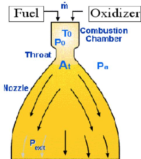
$$T_{exit} = \frac{T_0}{1 + \frac{(\gamma - 1)}{2} M_{exit}^2} =$$
