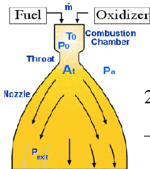
$$(I_{sp})_{ideal} = \frac{C^*}{g_o} \left[ \gamma \sqrt{\frac{2}{\gamma - 1}} \left( \frac{2}{\gamma + 1} \right)^{\frac{\gamma+1}{(\gamma-1)}} \right] =$$
