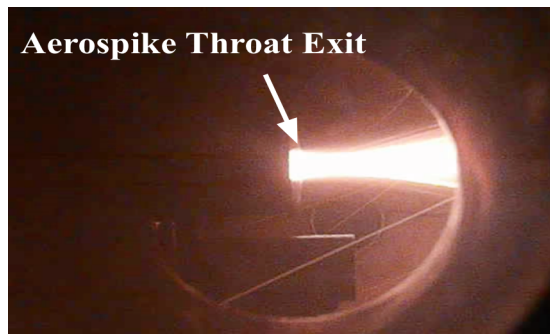
Figure 22. Exhaust Plume Images from Vacuum Tests of 8.5:1 Expansion Ratio Aerospike Nozzle.
