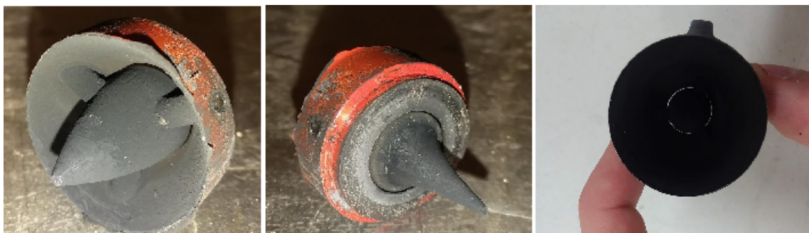
Figure 17. Intact Carbon-Throat Aerospike at Completion of Ambient Testing.
