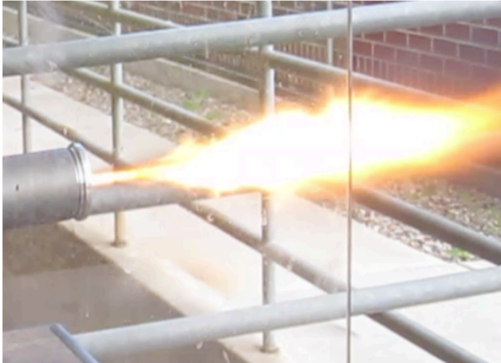
(a) Over-expanded Conical Nozzle Exit Plume.
