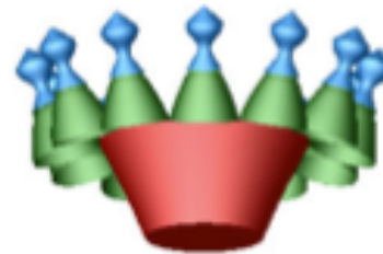
NOFB37 12 x 500 lbf (6000lbf) Monopropellant Engine
