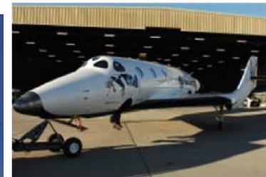
Virgin Galactic VSS Enterprise Powered by SNC Hybrid Rocket Motor
