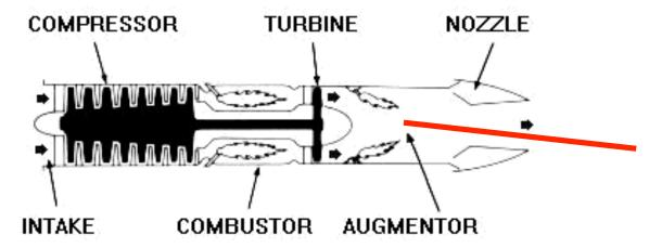
• ... that is why afterburners work ... left over  $O_2$  after combustion
