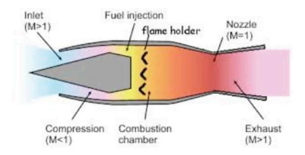
Ramjets cannot produce thrust at zero airspeed; they cannot move an aircraft from a standstill. A ramjet powered vehicle, therefore, requires an assisted take-off like a rocket assist to accelerate it to a speed where it begins to produce thrust.
