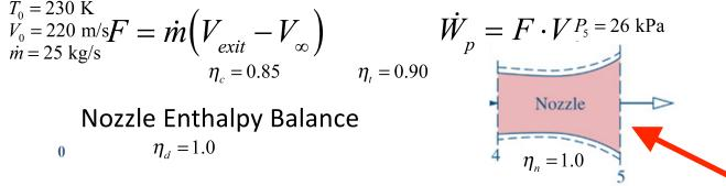
$$\dot{m}\left(h_4 + \frac{V_4^2}{2}\right) = \dot{m}\left(h_5 + \frac{V_5^2}{2}\right) = \dot{m}\left(h_{exit} + \frac{V_{exit}^2}{2}\right) \rightarrow V_4 \approx 0 \rightarrow V_{exit} = \sqrt{2\left(h_4 - h_{exit}\right)}$$
