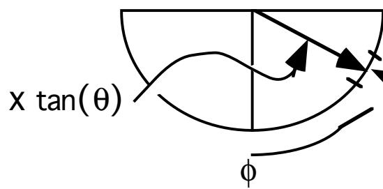
$$L_{\text{lower}} = \int_0^L \int_{-\frac{\pi}{2}}^{\frac{\pi}{2}} (p_{\text{cone}} x \tan(\theta_{\text{cone}}) \cos(\phi) d\phi) \cos(\theta_{\text{cone}}) \frac{dx}{\cos(\theta_{\text{cone}})} =$$
