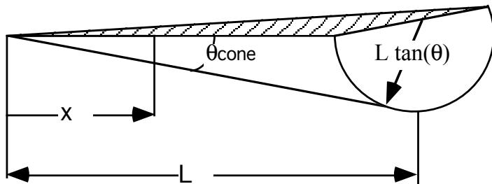
Axial Pressure force on Lower Cone Surface
