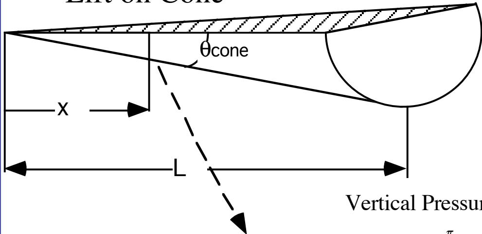
Vertical Pressure Force on Lower Cone Surface
