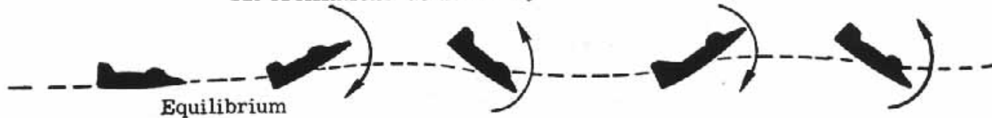
(b) Statically stable; neutral dynamic stability.
