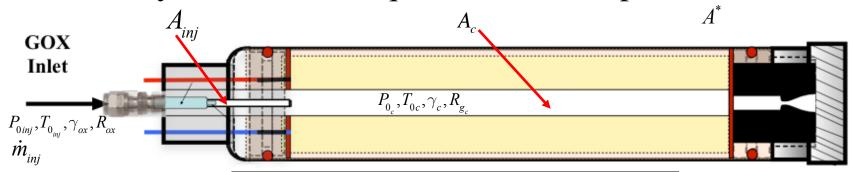
$$Subcritical: \left(\frac{P_{\text{0inj}}}{P_{\text{0}_c}}\right) < \left(\frac{\gamma+1}{2}\right)^{\frac{\gamma}{\gamma-1}}$$
