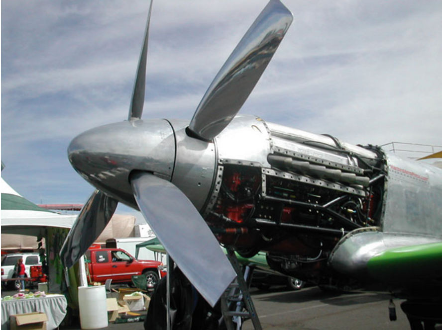
Fig. 4.29 Contra-rotating propellers on a Rolls-Royce–Griffon–powered P-51 unlimited racer
