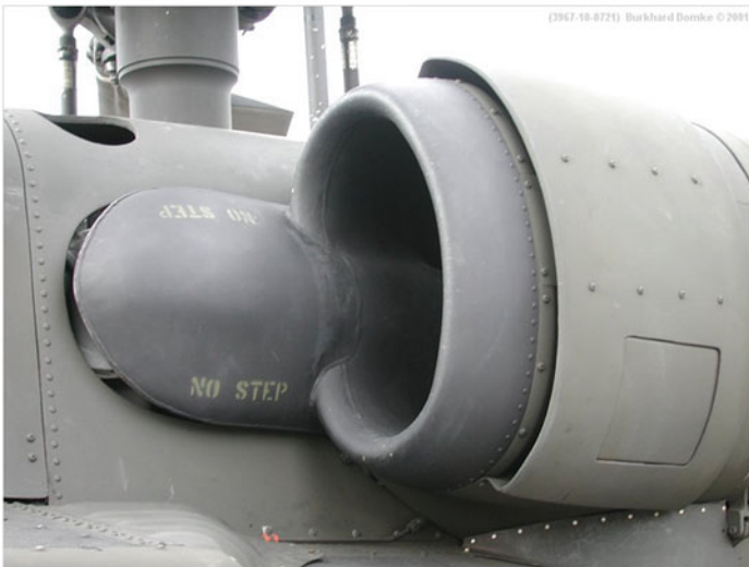
Fig. 8.32 Sikorsky UH-60 helicopter powered by two-side turboshaft engines
