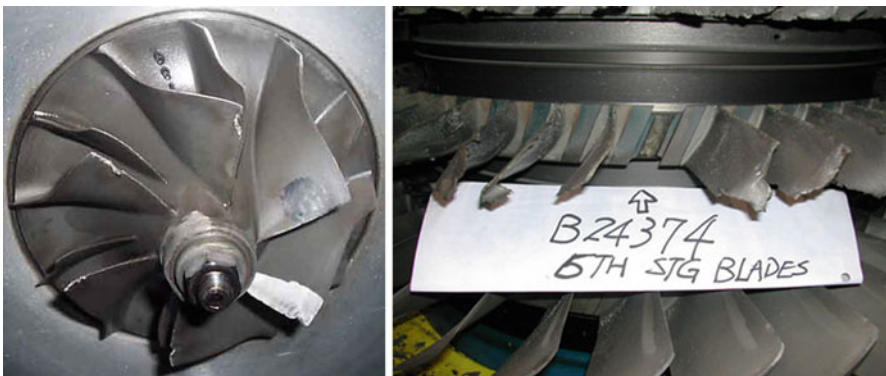
Fig. 9.36 Damaged blades of centrifugal compressor ( left ) and axial compressor ( right )
