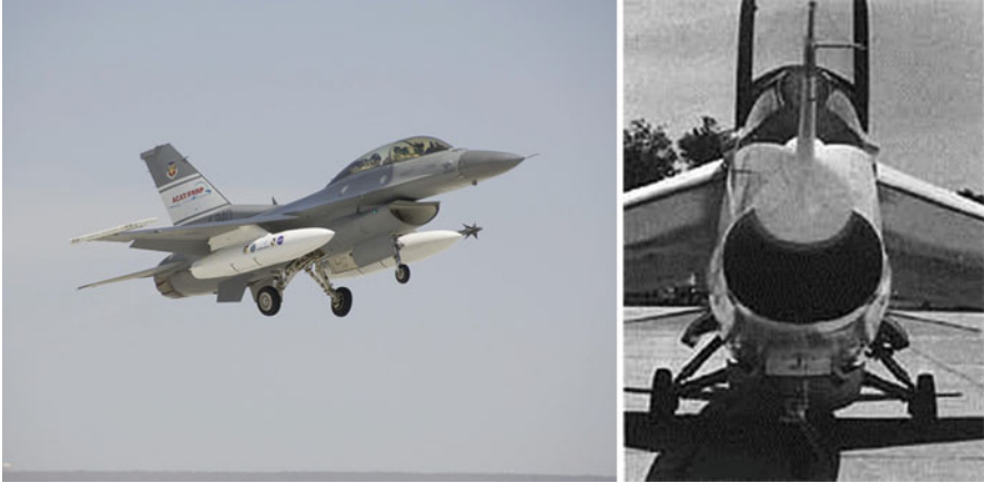
Fig. 8.26 F16 aircraft fitted with underslung intake
