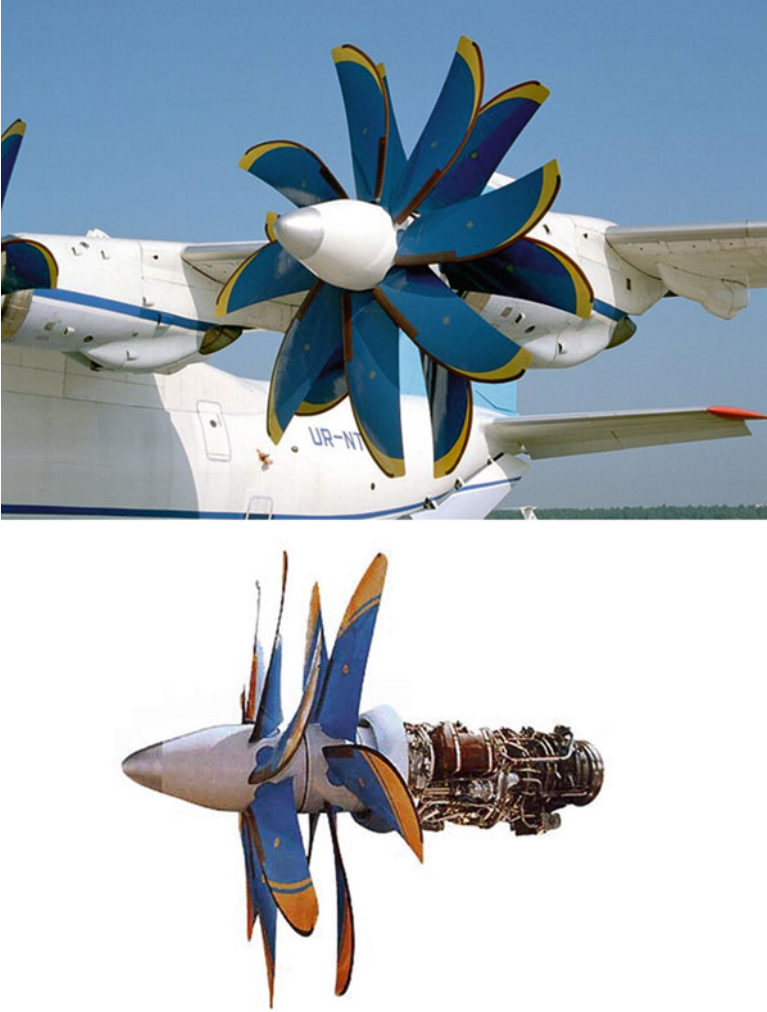
Fig. 7.25 AN-70 aircraft powered by tractor-type contra-rotating propfan
