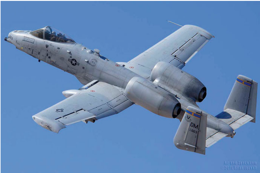
Fig. 8.27 Fairchild A 10-A Thunderbolt II aircraft with 2 engines installed to the empennage
