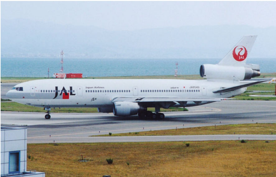
Fig. 8.8 DC-10 Combined wing and tail (3 engines pod installation)
