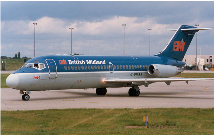
Fig. 8.6 DC-9 (fuselage 2 engines pod installation)
