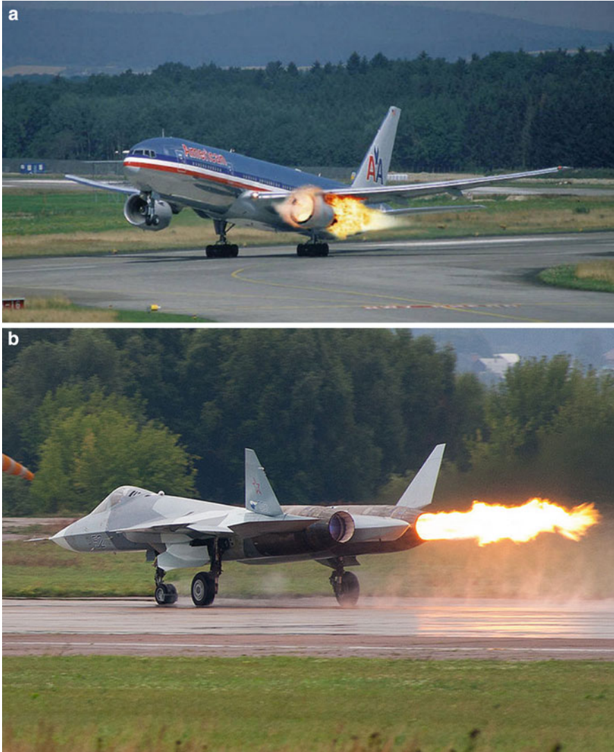
Fig. 9.35 Compressor surge leading to a flameout: (a) Boeing 777 aircraft; (b) Sukhoi T-50 PAK FA
