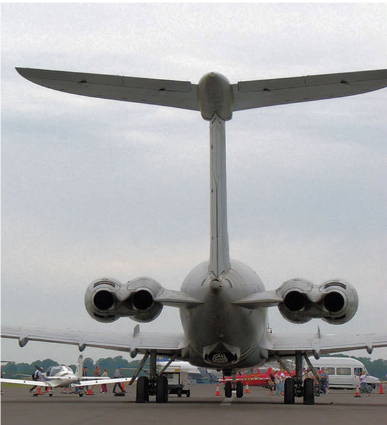
Fig. 8.7 Super VC-10 (4 engines fuselage pod installation)
