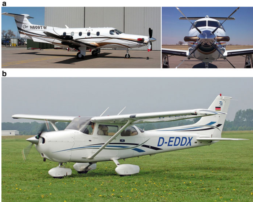
Fig. 8.15 Nose-mounted engines: (a) Pilatus PC-12 powered by a Pratt & Whitney Canada PT6A-67B turboprop and (b) Cessna 172 powered by one Lycoming IO-360-L2A four cylinder, horizontally opposed aircraft engine
