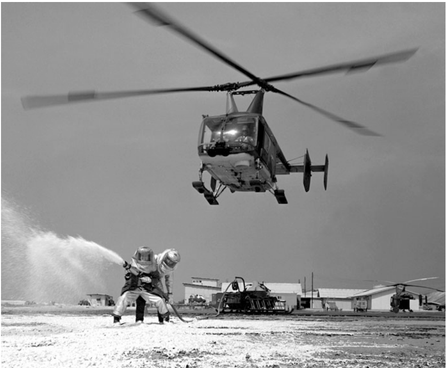
Fig. 1.42 HH-43 Huskie with intermeshing rotors
