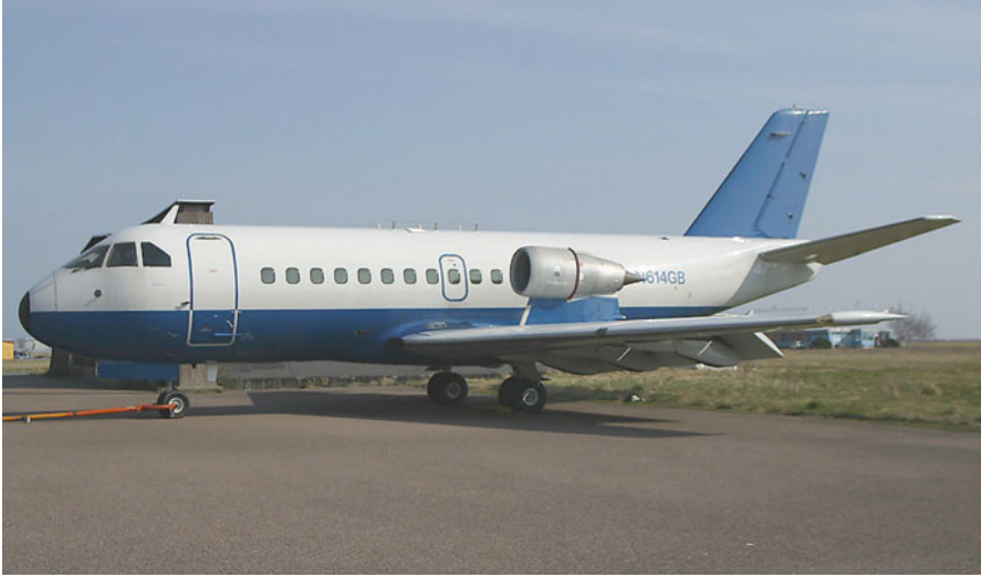
Fig. 8.4 Fokker VFW614 (2 engines above-wing installation)
