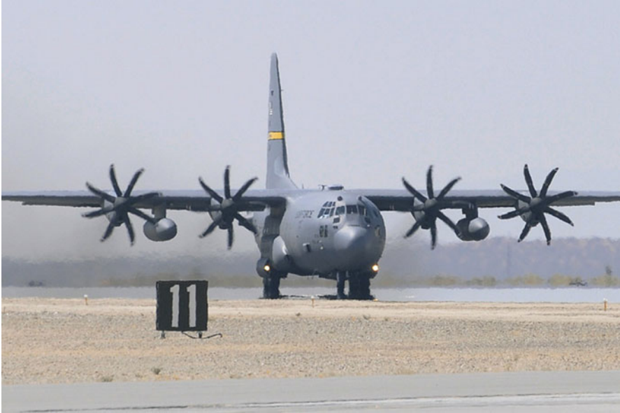
Fig. 4.34 Hamilton Sundstrand 8-blades NP2000 Propeller for C-130 aircraft
