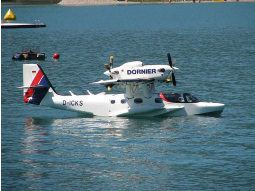
Fig. 8.14 Dornier Seastar powered by two push–pull turboprop above-wing installation
