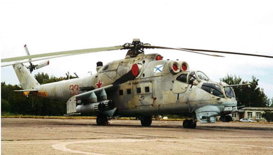
Fig. 8.31 Mi 24A (two engines above cabin with front intake)
