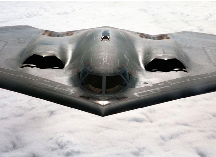
Fig. 8.29 B-2 Spirit Stealth Bomber with 4 engines having wing top intake
