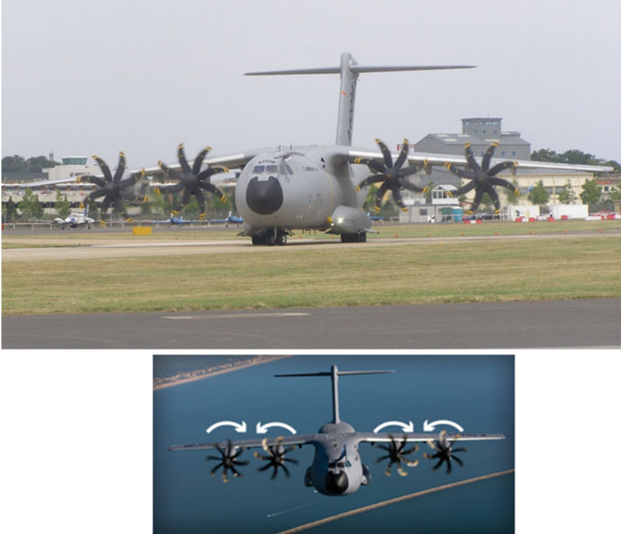
Fig. 4.30 Airbus A400 M aircraft (pair of propellers on each wing turn in opposite directions )
