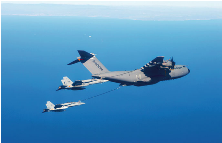
Fig. 1.33 Airbus A400M refueling a Spanish Air Force F/A-18 Hornet (Reproduced by permission from AIRBUS)
