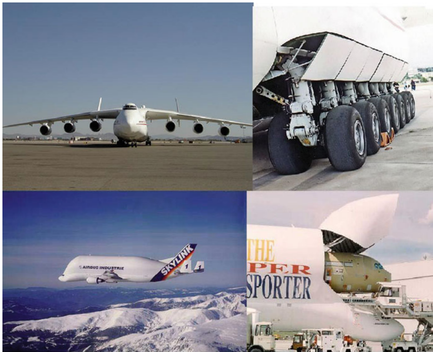
Fig. 1.17 Cargo Aircrafts (Freighters) Top: An-225 and Bottom A300-600ST, Reproduced by permission from AIRBUS
