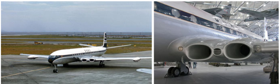
Fig. 8.2 De Havilland Comet (4 engines buried in the wing)
