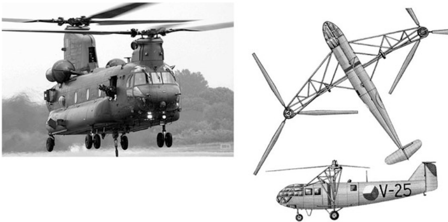
Fig. 1.40 Tandem rotor (CH-47 Chinook) and transverse rotor (Focke-Achgelis Fa 223)
