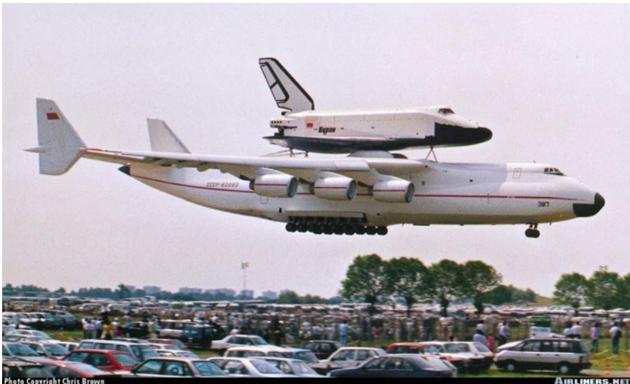
Fig. 8.3 Antonov An-225 (6 engines pod installation to wing)
