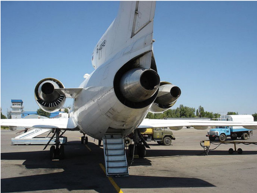
Fig. 8.10 Yak-42D (3 engines, pod installation; 2 fuselage and one tail)
