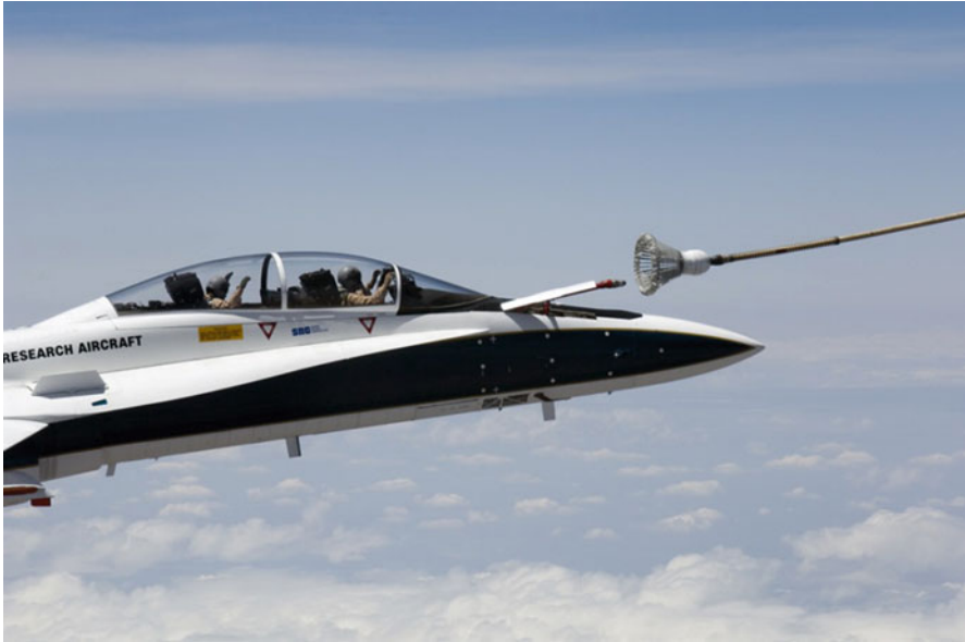
Fig. 2.5 Aerial refueling using the hose-and-drogue system
