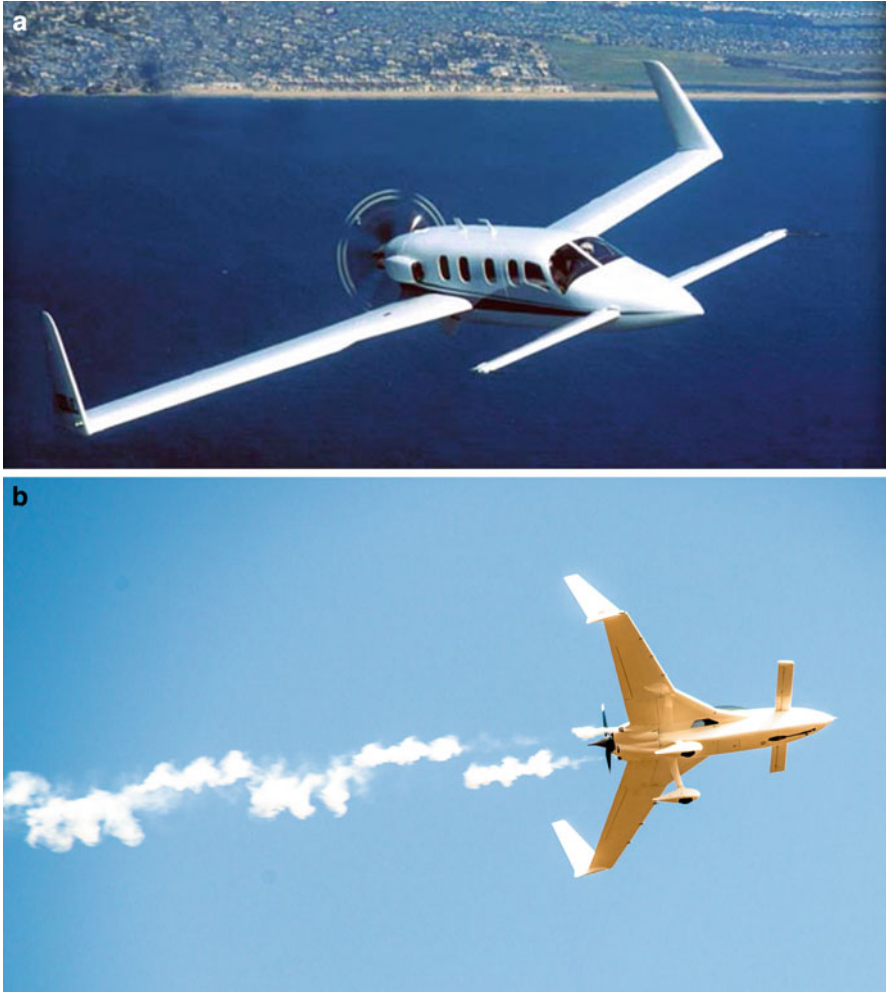
Fig. 8.16 Empennage installation: (a) Jetcruzer 500 driven by a single pusher-type turboprop engine and (b) Rutan Long-EZ powered by Lycoming O-235 piston engine
