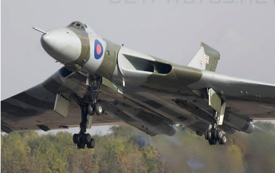
Fig. 8.28 Vulcan B-2 Bomber with 4 engines installed at wing root
