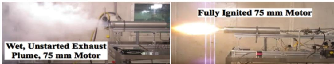
Figure 10: Comparison of wet and fully-started combustion exhaust plumes.
