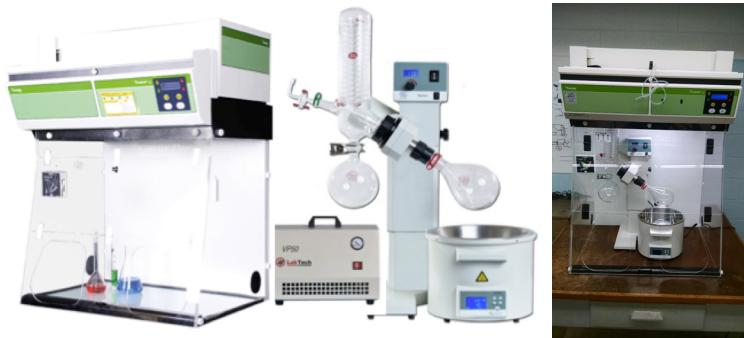
**Figure 4: Rotary evaporator and fume hood used to produce high concentration peroxide solution.**
