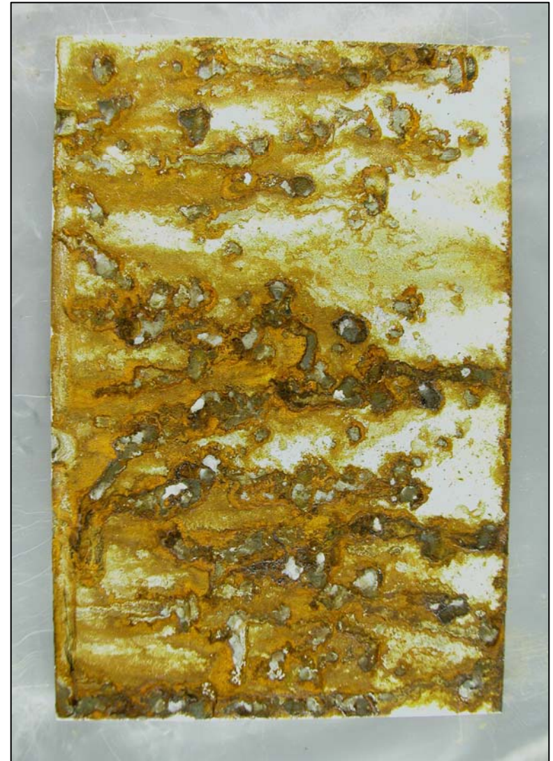
Unpassivated 410 coupon, sample #65
